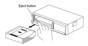
Pull the tray removal knob with your finger and draw the disc tray out of the magazine. Pay attention to the disc's signal surface when removing discs. (See "PRECAUTIONS" on page 4.)
