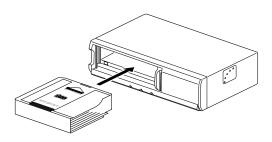
**5** After inserting the magazine, grasp the tab of the sliding door and slide the door all the way to the left until it locks with a "click."
